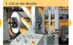
The incoming goods inspection of the coil is performed when it is put on the decoiler
