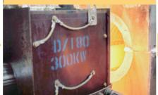
Heat treatment is performed online – in an inductive solution annealing process followed by a rapid cooling
